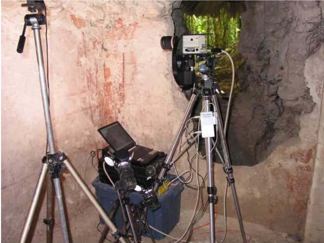
Figure 35. View of multispectral imaging equipment set in Room 1 La Sufricaya Str. 1 in front of mural 1 and 3 walls.
