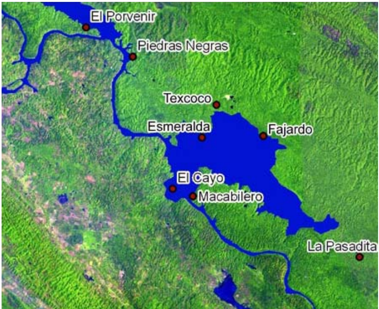
Figure 2. Model showing the impact of flooding resulting from a 46 m dam at the Boca del Cerro, Tabasco, México (by Todd Berendes, University of Alabama-Huntsville).
