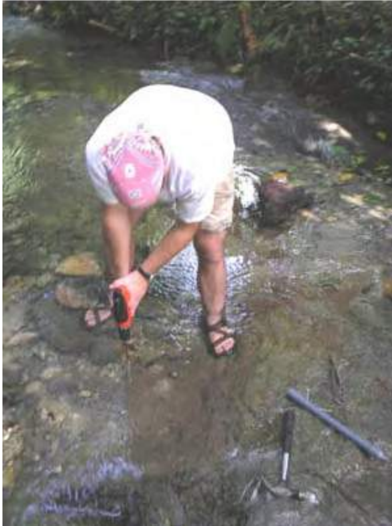
Figure 11. Kirk French drilling the holes in streambed for PT-1 with extended drill bit.
