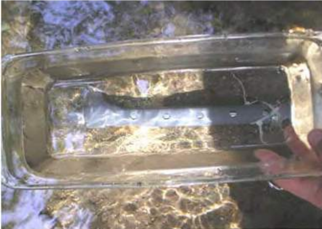
Figure 10. Viewing the anchored pressure transducer through a glass cooking dish.
