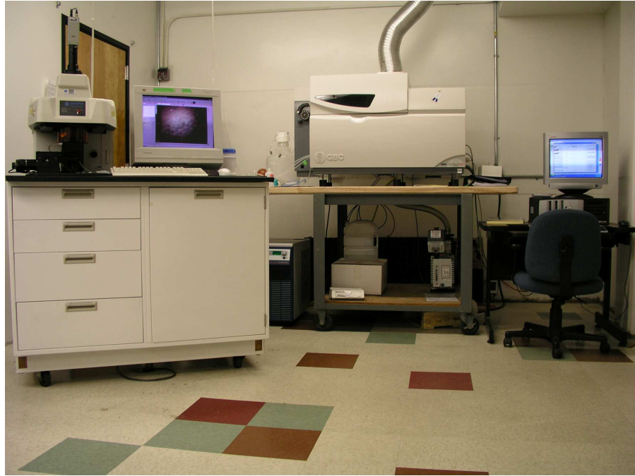
Figure 2. Laser Ablation Inductively Coupled Plasma Mass Spectrometer (photo by J. Dudgeon).
