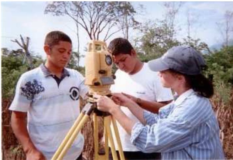
Figure 12. Pamela Geller teaches Carlos Alfredo Arito and Carlos Jose Torres Lopez to set up the total station.
